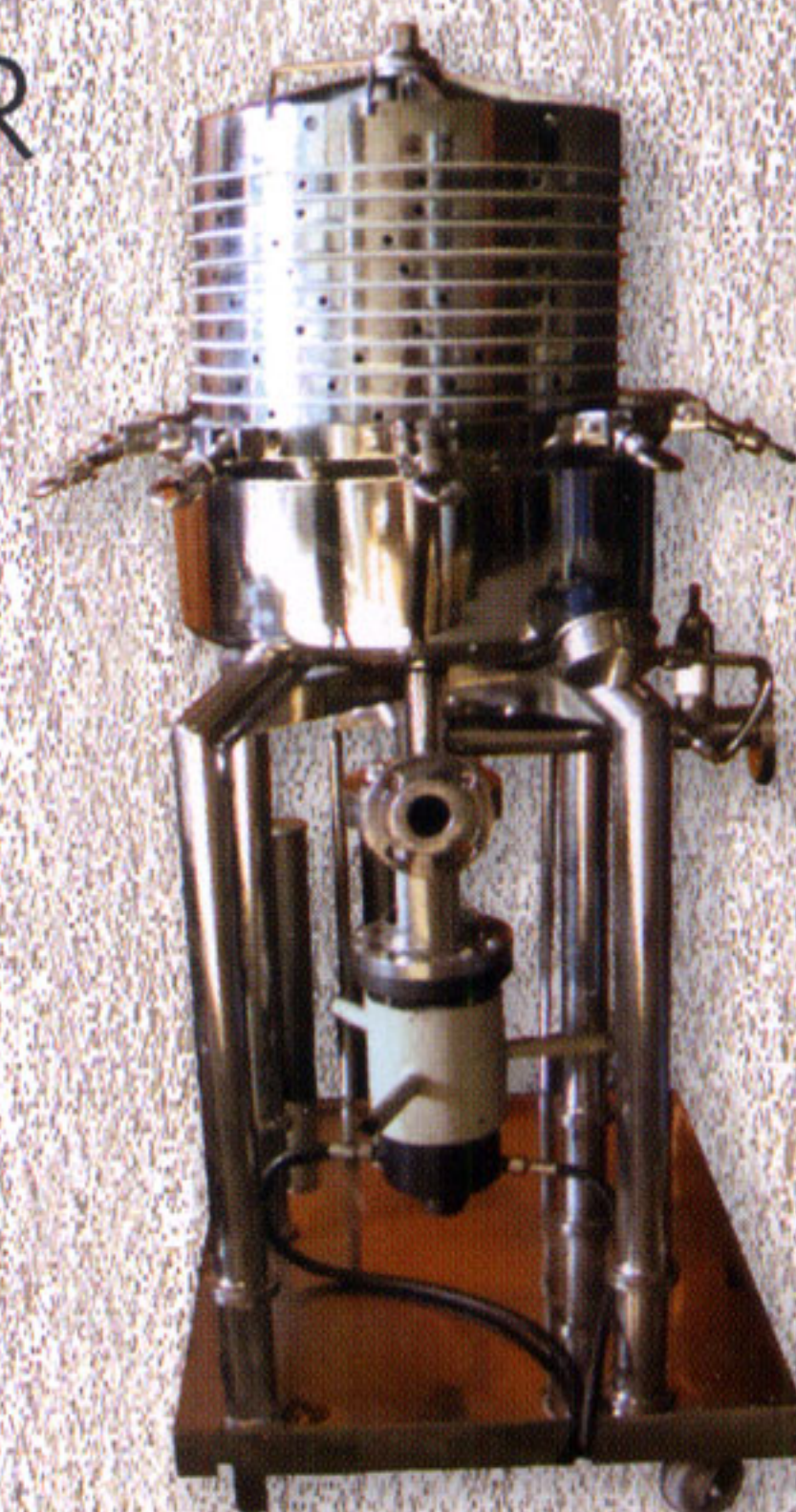
Zero hold up Horizontal Plate Closed Filter with Hydraulic tightening
